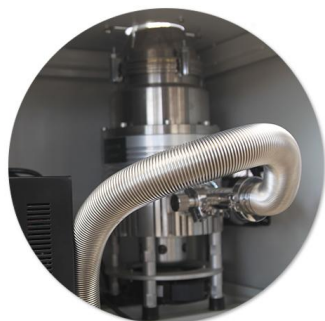
High Vacuum Molecular Pump - ultimate vacuum 0.05Pa
